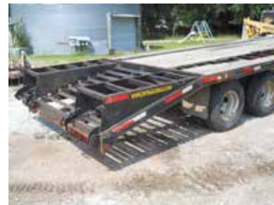
EW Flat Bed Trailer w/ Ramps. Floor needs replaced, one jack is bent, Double Axel w/ Duals, Pintle hitch, 20' Bed w/ 5 1/2' Dove Tail, Good Rubber
