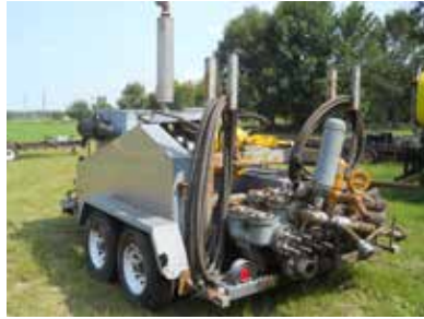
Mod. 3176 Gaso Mud Pump w/ Cummings Engine, Evco Power Swivel
